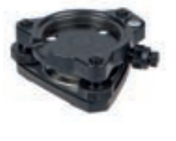
Ref.-No. 482 100 Tribrach with optical plum- met, universal 5/8" base plate with forced-centering locking and optical plummet. Colour: black
