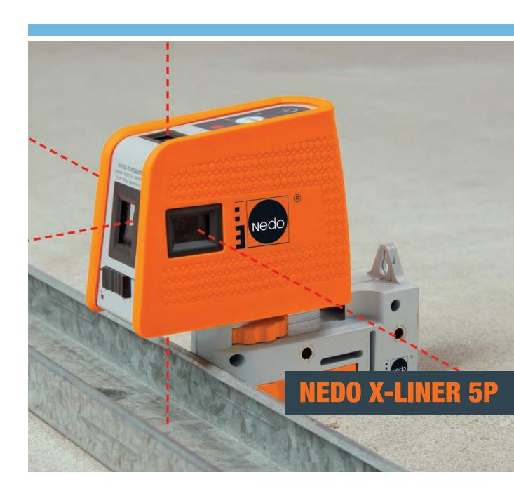
Easy, single-button operation. Reliable, magnetically damped pendulum for precise results. The device selflevels automatically on inclines of up to 4° so that the laser points from the X-Liner 5P are always projected exactly vertically or horizontally.
